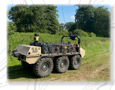
Convoy – lock onto a human driven vehicle and follow at up to 30 km/h
